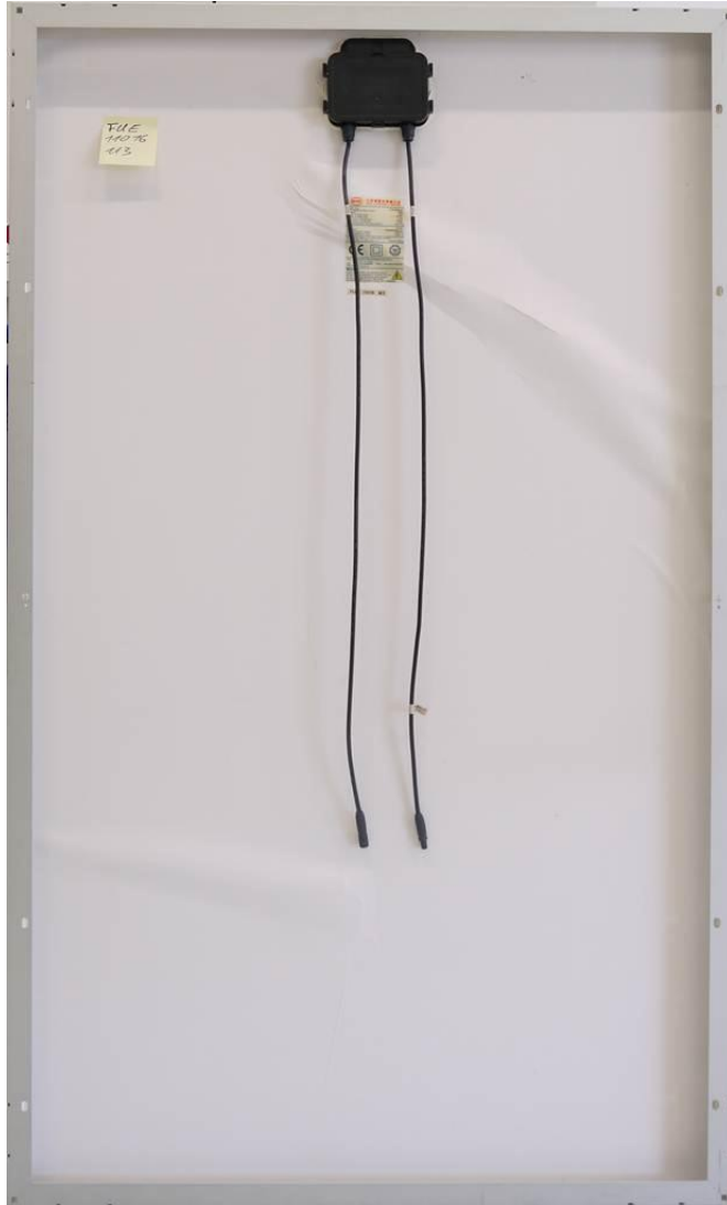
Fig. 2 M3 strong backsheet delamination
